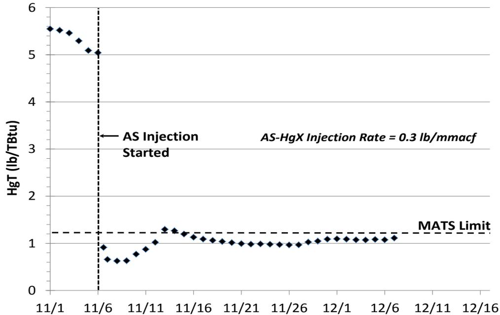
Figure 2. Results from the extended trial of AS-HgX at Neil Simpson 2.
