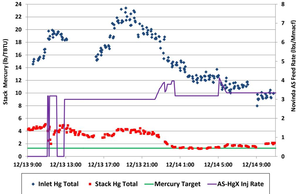
Figure 3. Stack mercury measurements from Confidential Plant 1.
