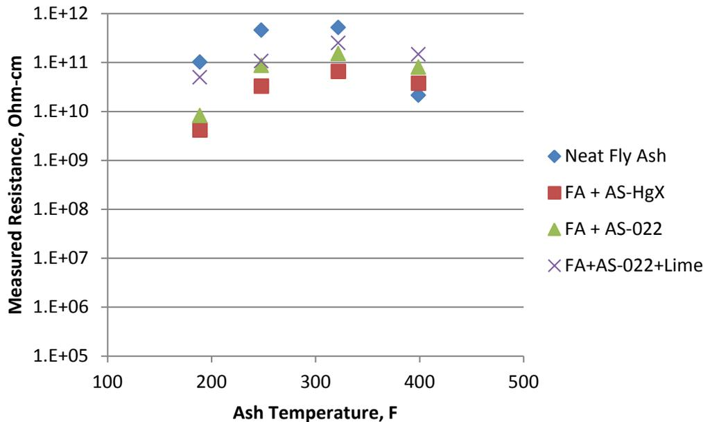
Figure 5. Resistivity test results from Confidential Plant 3.
