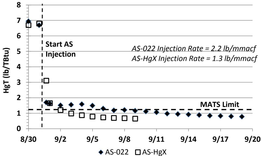
Figure 1. Results from Wygen 2 injection trials of Amended Silicates.
