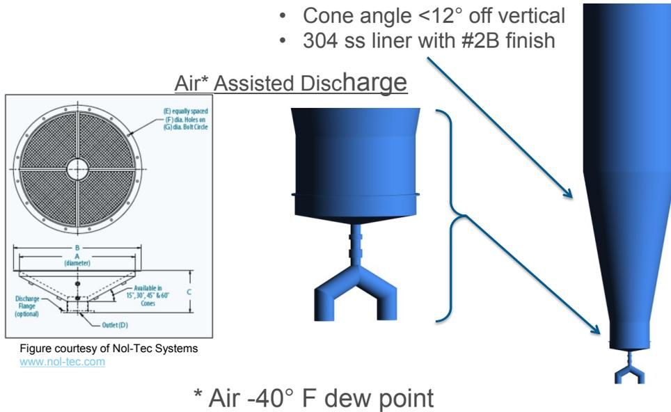
Figure 1 Flexible feed hopper design
