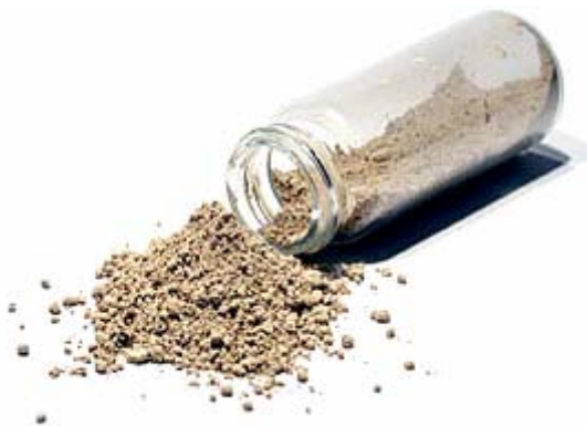
Figure 1. Amended Silicates™ is a non-carbon, mercury-specific adsorbent.
